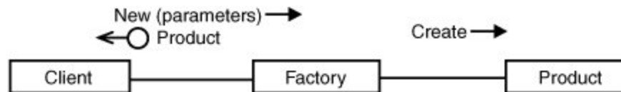
Figure 2-7. An instance diagram for the Factory pattern
