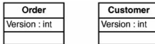
Figure 8-2. Added Version fields to some of the Aggregate roots
